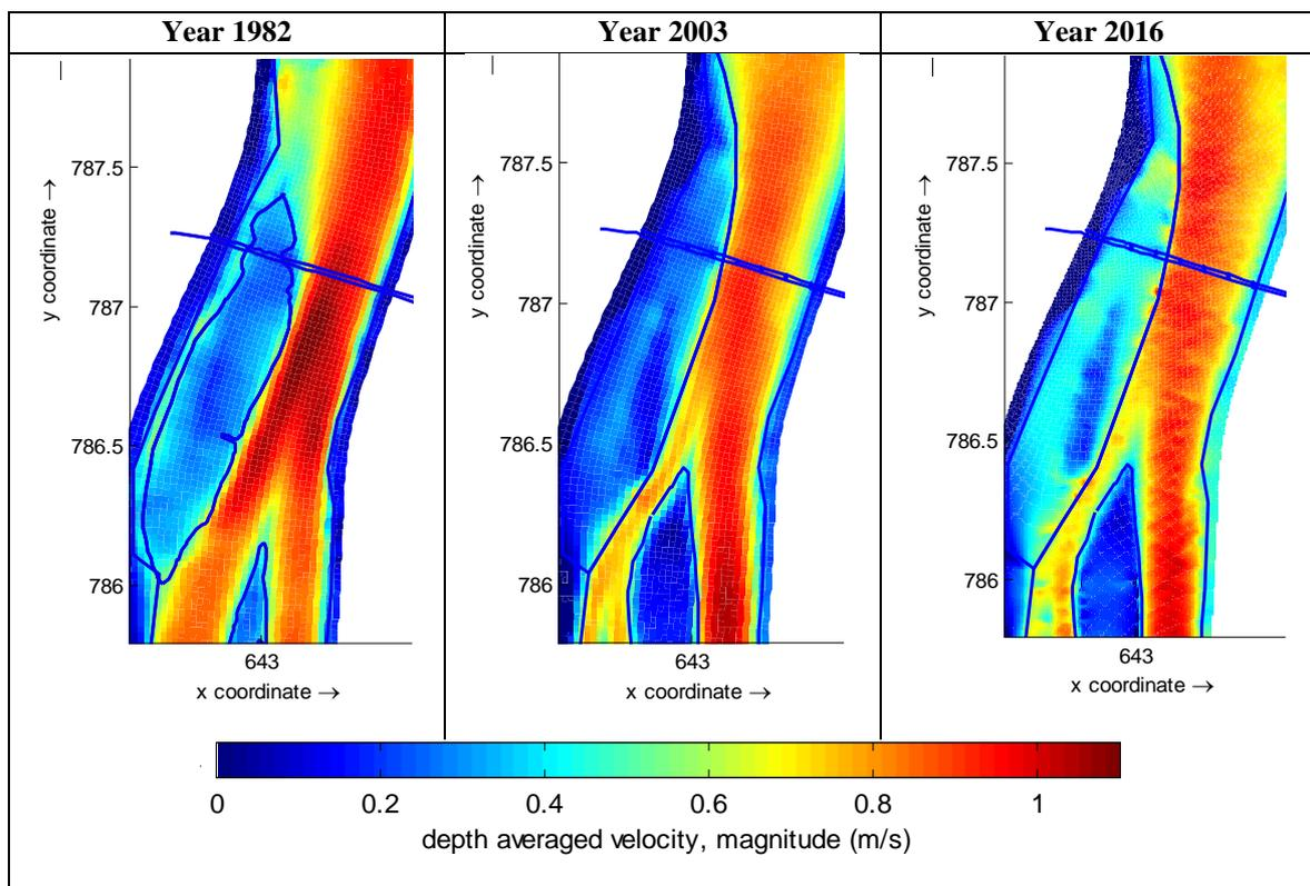
Figure 9: Depth average velocity at maximum flow at the three years
