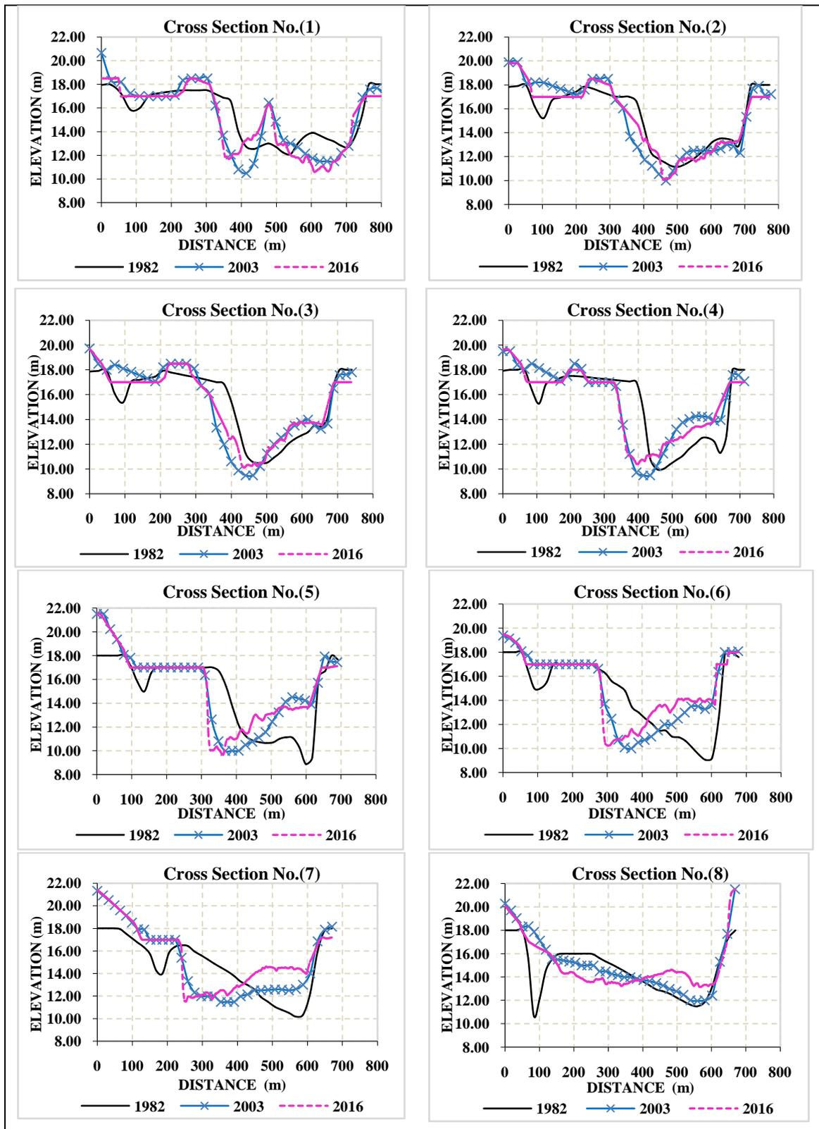
Figure 7: Comparison between the bed elevation at three years 1982, 2003 and 2016
