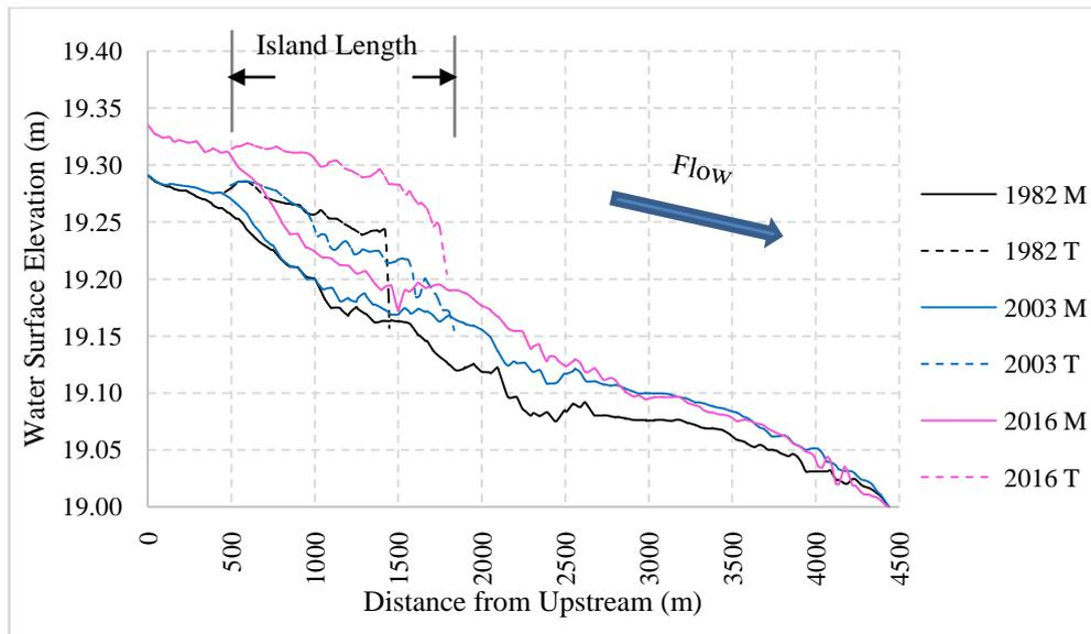
Figure 8: Water surface slope at the deepest points along the reach at the three years in maximum flow, M (main channel) & T (tributary channel)
