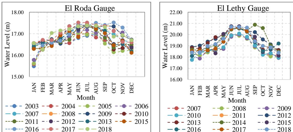
Figure 2: River Nile hydrograph for W.L at El Roda and El Lethygauges
