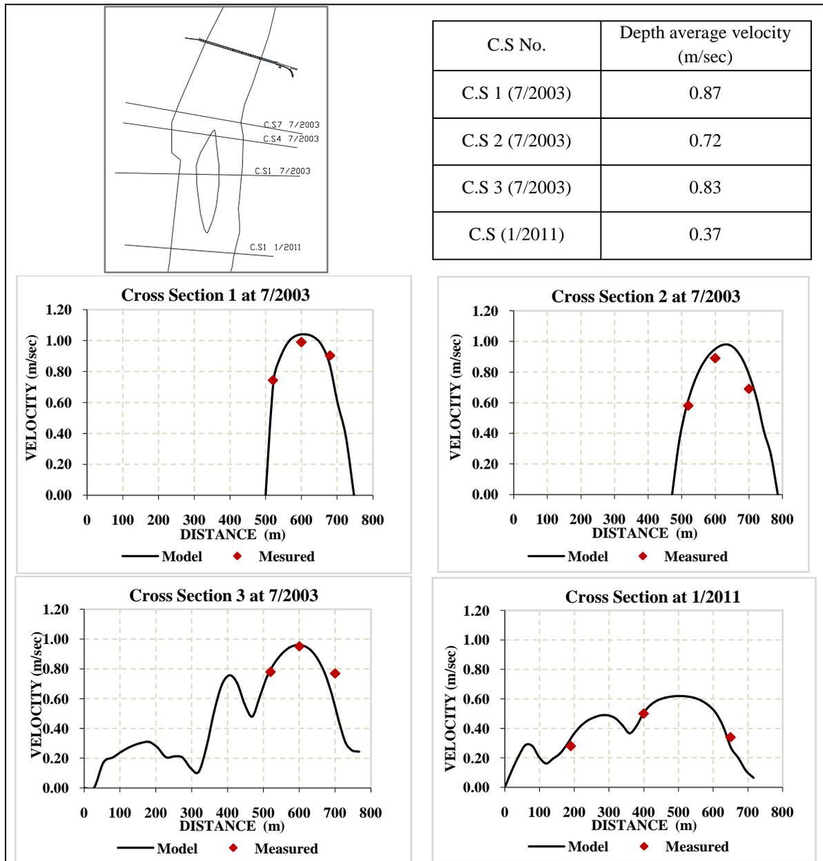
Figure 5: Depth average velocities calibration and the cross sections location
